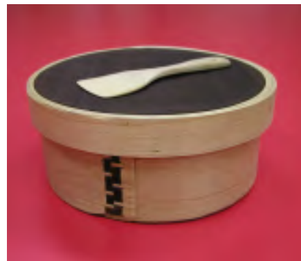
ABOVE Sieve and paddle used to strain wheat starch paste. CLOCKWISE FROM BELOW RIGHT Brushes used to attach mounting materials, apply water, and tamp paper layers together.
