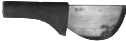
Conservators usually use a “round knife” to cut paper and silk.
